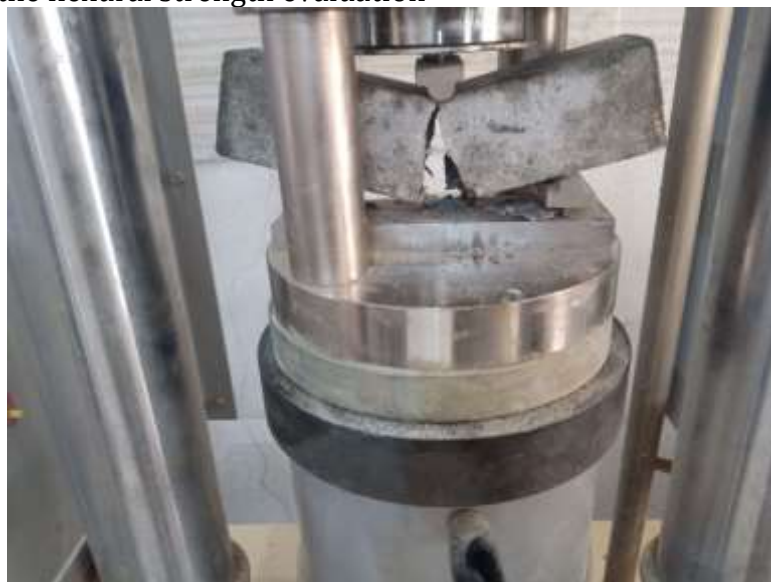
Figure(3): flexural strength test
