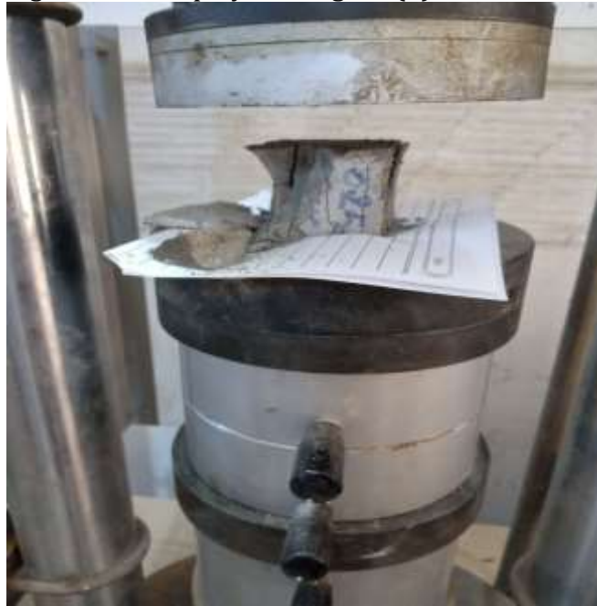
Figure(2): compressive strength test
