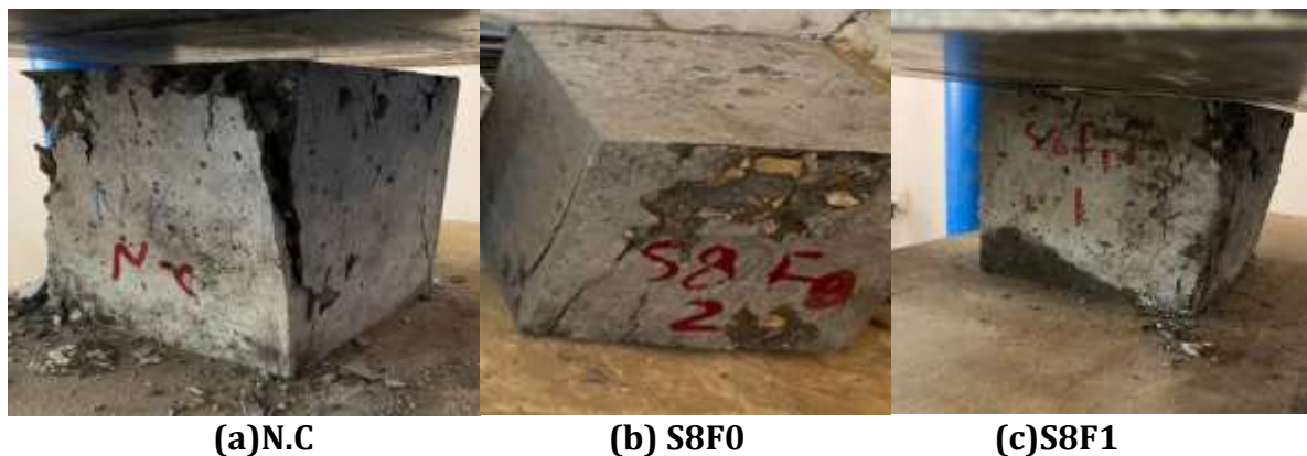
Figure (13): (a),(b) and (c) , crack pattern of cubics (compressive strength) of N.C, S8F0 and S8F1
