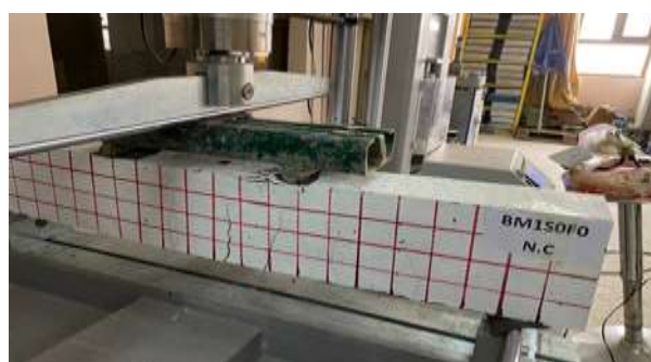
Fig17 : Cracks Pattern of N.C
