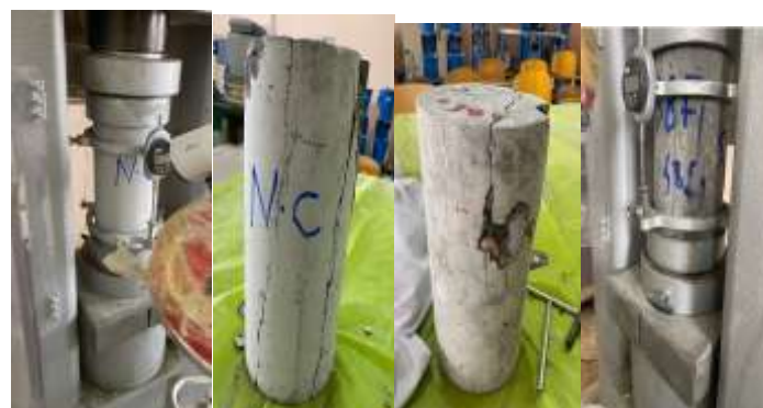
Fig.15: Comparison of the crack pattern N.C , S8F0 and S8F1 of cylinders
