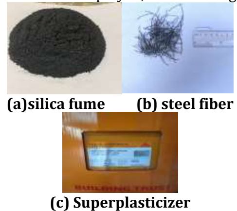
Fig.4: Hooked-end fiber , silica fume and Superplasticizer used (a) and (b)
