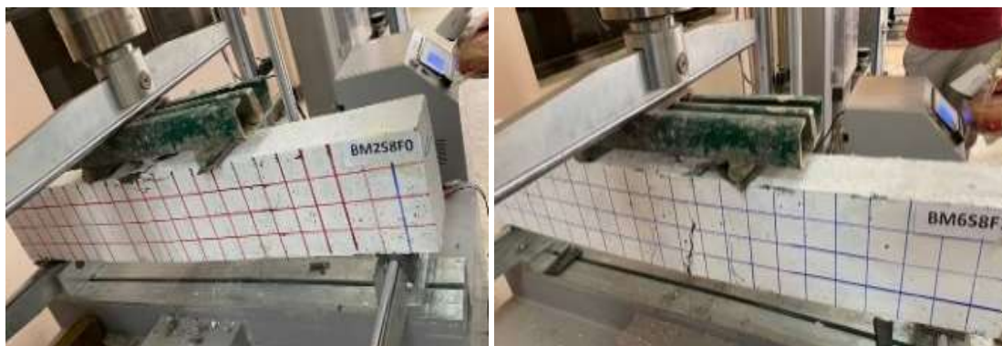
Fig.20 : Cracks Pattern of S8F0 and S8F1
