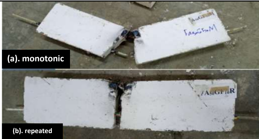
Figure.8. (a) Bar rupture failure of GFRP-reinforced specimen (monotonic loading) (b) pull-out failure of GFRP-reinforced specimen (repeated loading)
