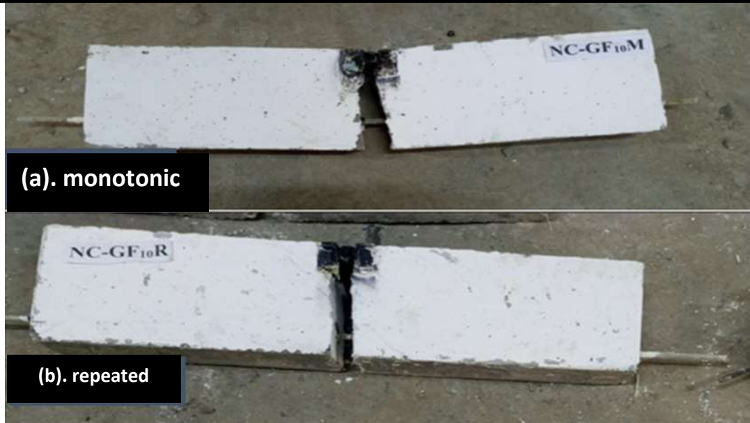
Figure.6. (a) pull-out failure of GFRP-reinforced specimen (monotonic loading) (b) pull-out failure of GFRP-reinforced specimen (repeated loading)
