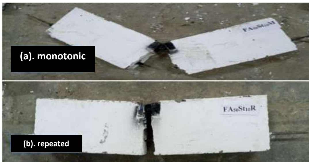
Figure .7. (a) pull-out failure of the steel-reinforced specimen (monotonic loading) (b) pull-out failure of the steel-reinforced specimen (repeated loading)
