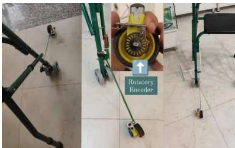
FIGURE1 : Modifying the Walker by Adding the Front Wheel and Potentiometer.
