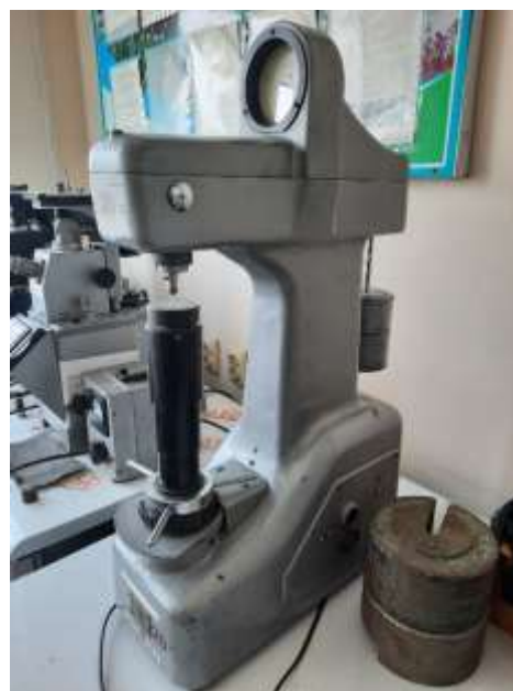
Figure 2. ZIP TK-2M Rockwell Press. Experiments
